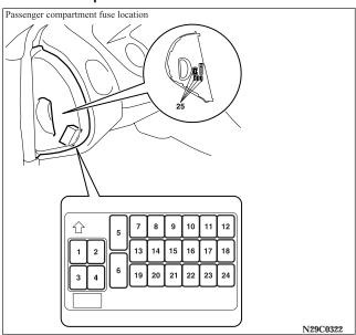
The fuse cover lists the names of the electrical systems and the fuse capacities. Spare fuses are contained in the
